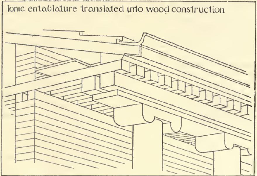
FIG. 22—IONIC ENTABLATURE, RETRANSLATED INTO WOOD. (AFTER DURM)
