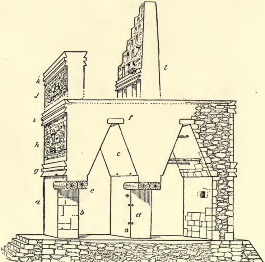
FIG. 283—TRANSVERSE SECTION OF A TYPICAL MAYA BUILDING.
