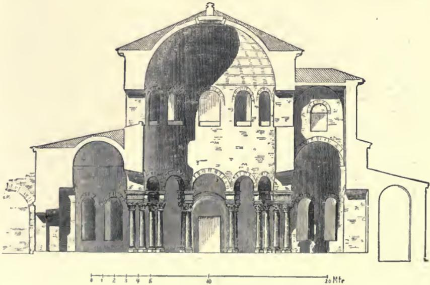
FIG. 71—ROME. SANTA COSTANZA. SECTION SHOWING THE CONSTRUCTION
